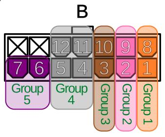
The 12 digital outputs are divided into five groups. Each group contains two outputs, except for Group 4, which has four. When configuring outputs, keep the following group-based limitations in mind:
